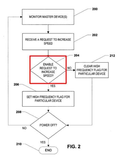
Appx1387. Figures 3, 4, 5, and 6 likewise depict a "decision step" of determining whether to grant the request—"Yes" or "No"—based on defined parameters (*e.g.*, whether the device is a "preferred device"). Appx250-51(6:1-7:19).
