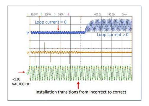
Appx21650. It depicts pulse signals in orange (middle line) and "loop current" in blue (top line). Appx10094(183:1-14; 185:18-186:2). It shows that the "loop current" remains zero—meaning the switch has *not* been turned on—until *after*
