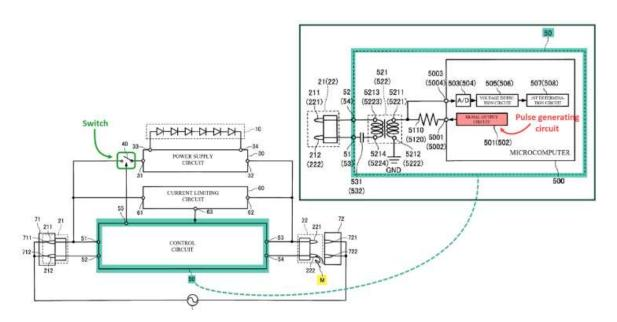
Appx21496. That is virtually identical to the LT2600 chips' structure—which Super omits. As in Ono, the pulse generating circuit is a *component* of a larger chip ("CP1") that is connected to a switch located on a separate chip ("CP2"):
