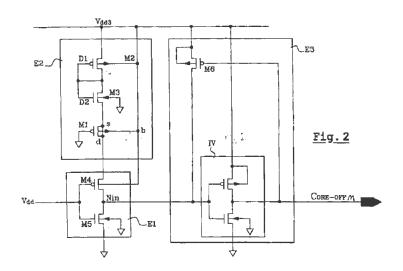
Figure 2 shows a detection device "compris[ing] an output stage E3 following the input stage E1, to obtain the desired output levels for the inverse detection signal  $C_{ORE-OFFn}$ ." Ex. 1008, ¶¶ 35–37.
