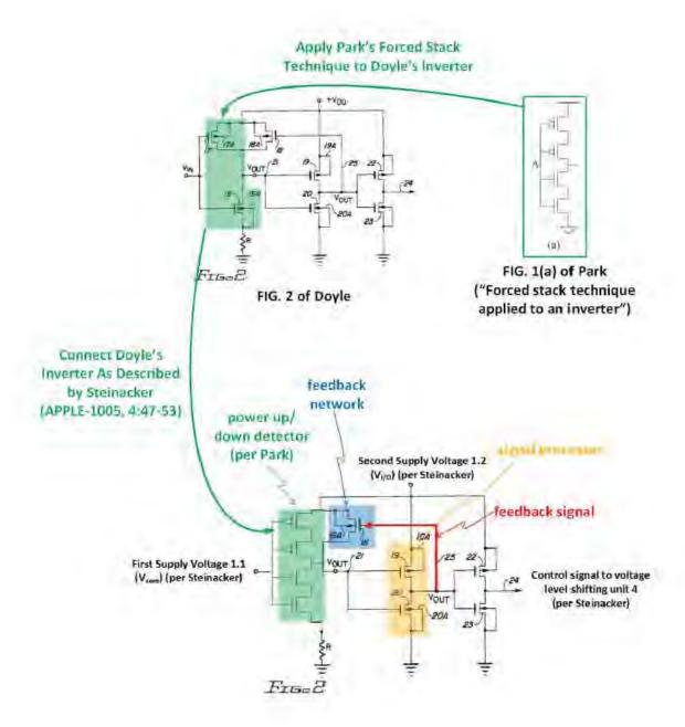
Pet. 20; 1316 Pet. 19. According to Petitioner, the figure reproduced above shows Park's Figure 1(a), which shows the forced stack technique applied to an inverter, Doyle's Figure 2, and a modified version of Doyle's Figure 2 showing the application of the forced stack technique applied to transistors 17 and 18. Pet. 20; 1316 Pet. 19.
