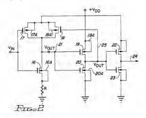
Id. at Fig. 2. Figure 2 "is a schematic circuit diagram of a self adjusting TTL [(transistor-transistor logic)] compatible input circuit according to the present invention." Id. at 3:35–37. According to Doyle, an "object of the invention [is] to provide a MOSFET circuit structure that, in effect, produces a MOSFET drain current having a predetermined amount or range of variation with respect to temperature and/or certain MOS processing parameters." Id. at 2:32–36.
