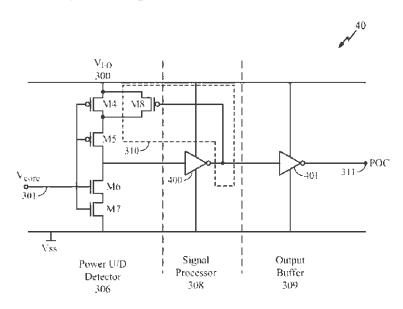
Figure 4 "is a circuit diagram illustrating another POC network configured according to the teachings of the present disclosure." *Id.* at 4:28–30. The '674 patent describes the operation of the feedback circuit in Figure 4 as follows:
