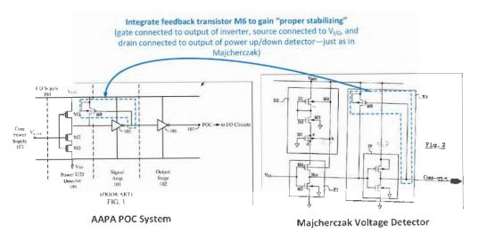
Pet. 44. The figure reproduced above shows Majcherczak's Figure 2 annotated by Petitioner (right) and a version of Figure 1 of the '674 patent (AAPA) modified by Petitioner to integrate the feedback transistor M6 from Majcherczak's Figure 2 (left). *Id.* Petitioner also provides a differently annotated version of its proposed combination as reproduced below.
