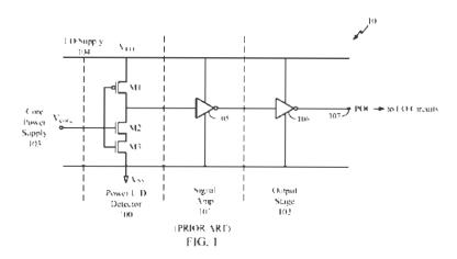
*Id.* at Fig. 1. "FIG. 1 is a circuit diagram illustrating a conventional POC system for multiple supply voltage devices" and is identified as prior art. *Id.* at 4:18–19, Fig. 1. According to the '674 patent, the POC "is made up of three functional blocks: power-up/down detector 100, signal amplifier 101, and output stage 102. Power-up/down detector 100 has PMOS transistor M1 and NMOS transistors M2-M3." *Id.* at 1:60–63.
