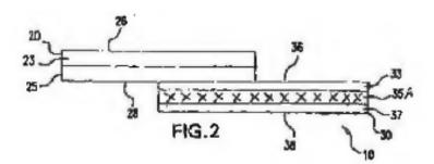
[Appx3305] WP's patent attorney claimed that this modified drawing demonstrated why the Shirrell '909 wrap failed—because the mesh being placed within a film layer caused delamination.
