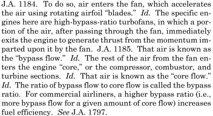
The compressor and turbine sections are further divided into high- and low-pressure segments. J.A. 1183. Each of the high- and low-pressure compressor and turbine sections consist of stages, or a "a matched set of rotating blades and stationary airfoils." *See Gen. Elec. Co. v. United Techs. Corp.*, No. IPR2017-00428, 2018 WL 3105491, at \*7 n.6 (P.T.A.B. June 22, 2018) (*Final Written Decision*); J.A. 1186. In the figure above, these stages are represented by
