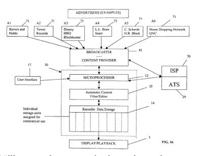
Figure 16 "illustrates the communication pathways between advertisers 71, a broadcaster content provider 41, and . . . . VPR/DMS 30." Ex. 1003, 30:60–63.
