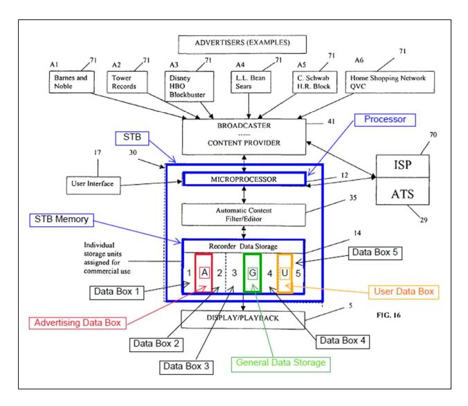
Appx418 (Fig. 16) (annotated to illustrate exemplary reservations of data boxes for different purposes). In the context of advertising data, the processor and software operate to store the non-advertising data in a separate section of memory (e.g., the "General Data Storage," or Data Boxes 1-5), and to prevent non-advertising data from being stored in the reserved section for advertising data, as illustrated above and indicated below.
