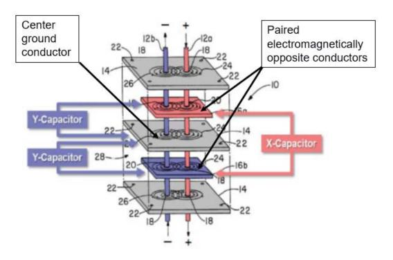
Appx373 (colors and annotations added). Among other things, the figure shows a center common ground conductor 14 (grey plane in the middle) positioned between and separating paired electromagnetically opposite conductors 16a and 16b (red and blue planes). Appx389-390 ('249 patent) at 16:5-29, 17:1-3, 17:43-57.
